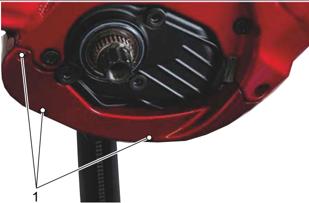
Figure 106: Attachment screws in lower motor cover (1)
