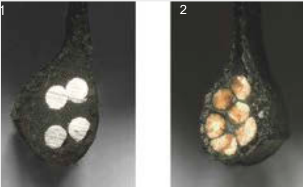
Figure 30: Steel bead core (1) and Kevlar bead core (2)
