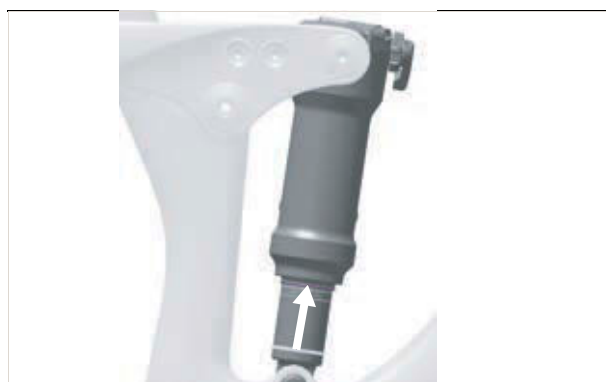
Figure 166: Moving the O-ring on the rear frame damper
