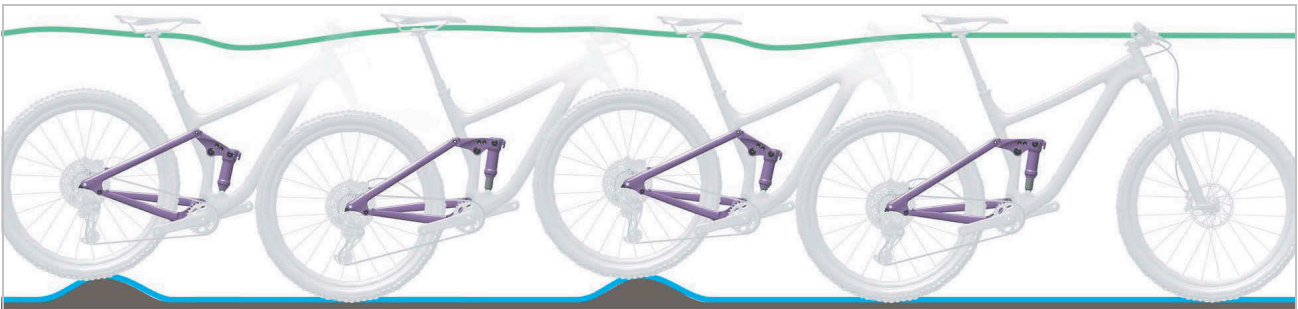
Figure 5: Optimum rear frame damper ride performance
