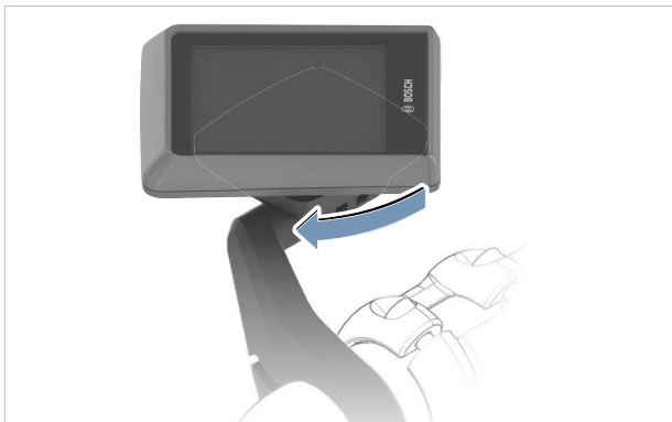
Figure 175: Turning the display clockwise
