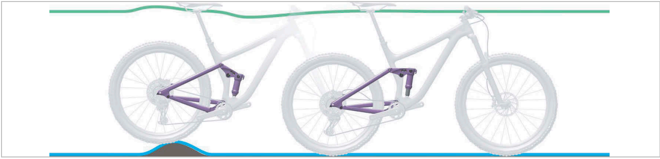
Figure 7: Optimum rear frame damper ride performance over bumps
