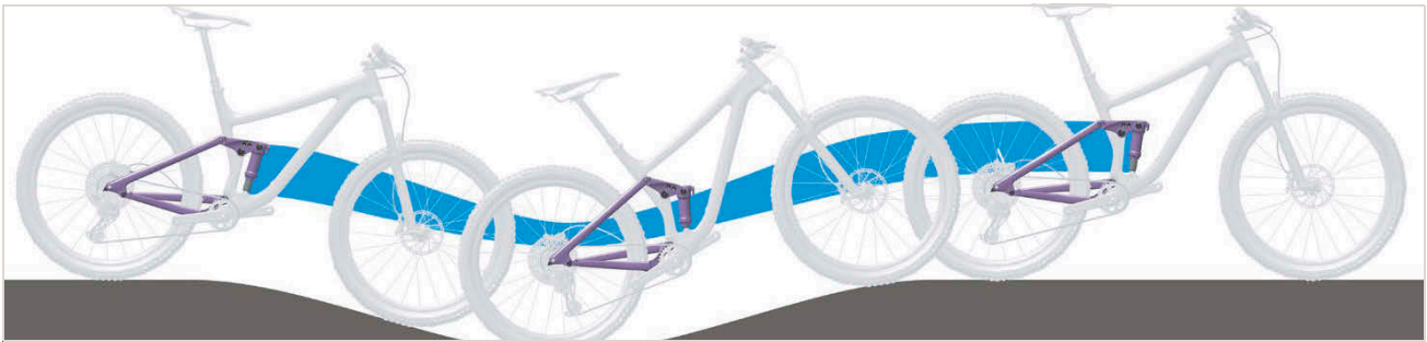
Figure 262: Excessively soft suspension in the rear frame damper on hilly terrain
