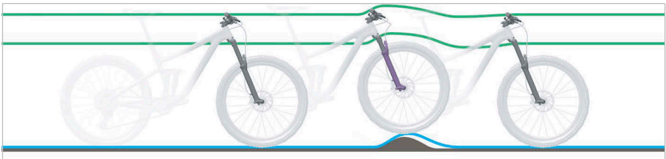
Figure 257: Excessively hard damping in the suspension fork on bumps
