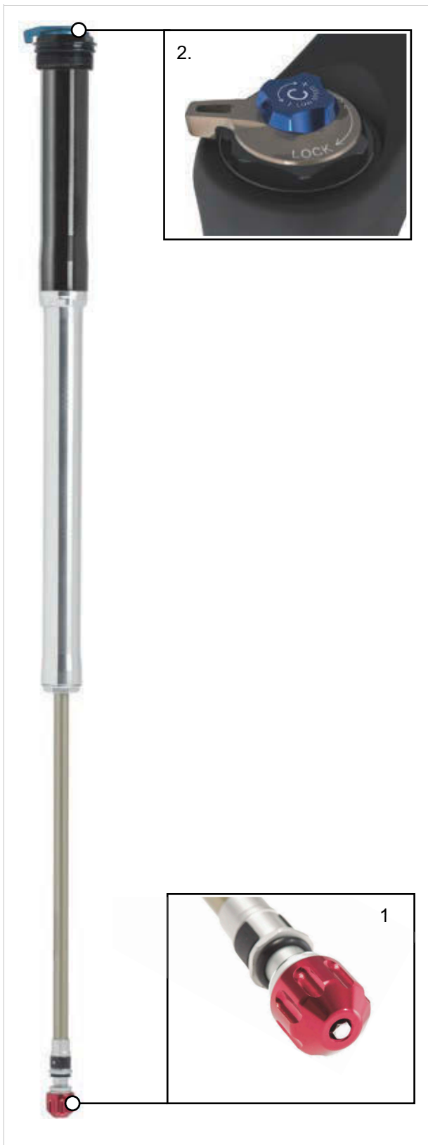
Figure 25: LOR operating elements
