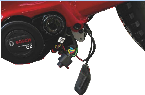
Figure 112: Motor without cover
