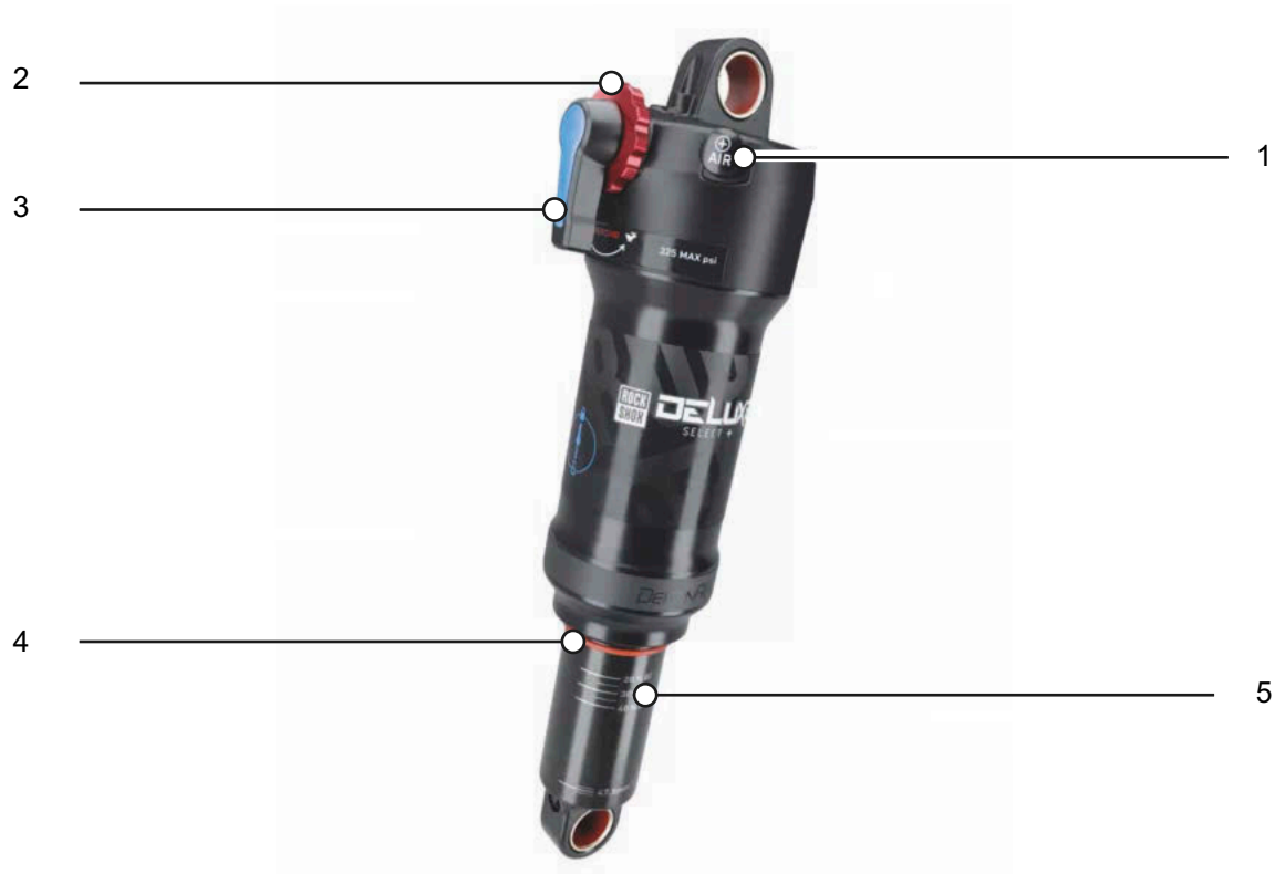
Figure 88: ROCKSHOX Deluxe Select rear frame damper structure design
