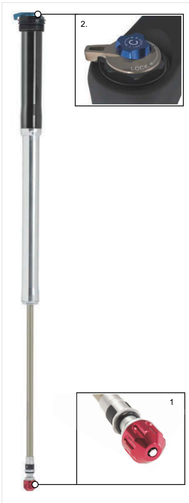
Figure 27: LORC-PCS operating elements
