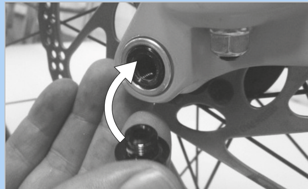
Figure 129: Inserting the securing screw
