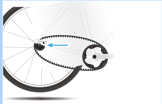
Figure 123: Pushing the rear wheel backwards
