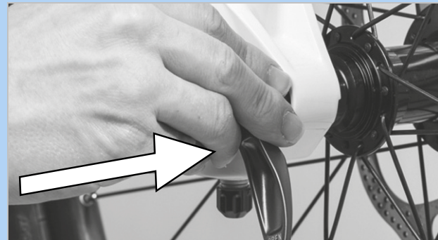
Figure 138: Inserting the quick release in the direction of the arrow
