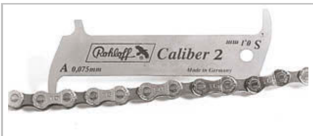
Figure 239: Example of a ROHLOFF gauge
