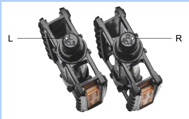
Figure 104: Example of mark on pedals
