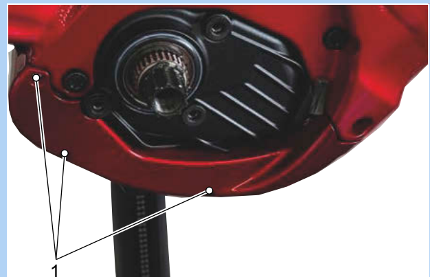
Figure 110: Attachment screws in lower motor cover (1)
