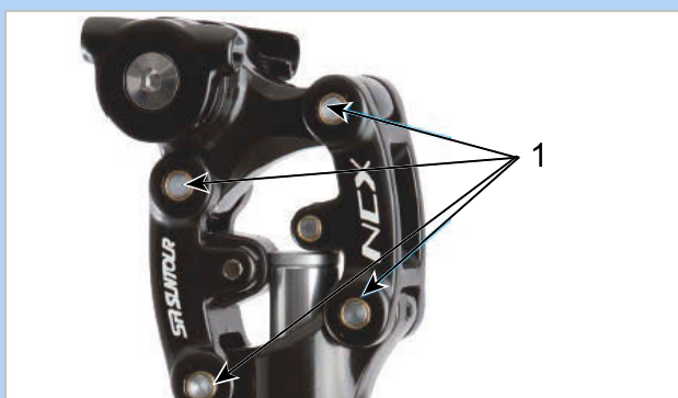
Figure 264: SR SUNTOUR suspension seat post lubrication points
