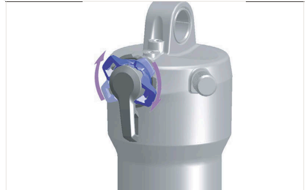
Figure 197: Adjust the compression adjuster so that it is harder
