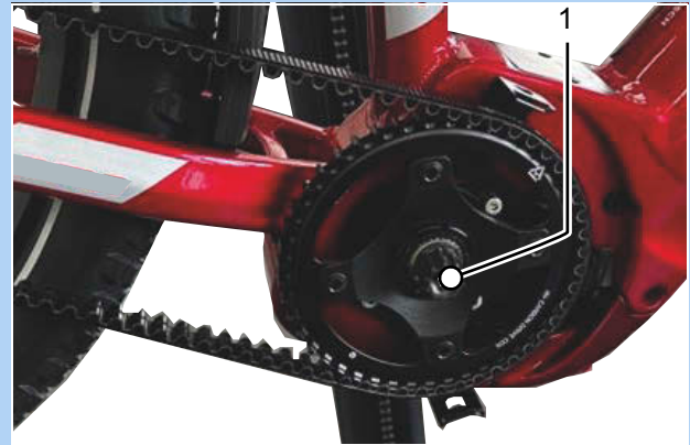
Figure 109: Unfastening the belt sprocket
