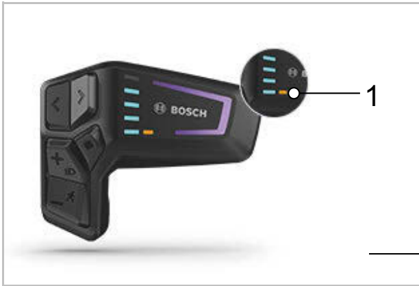
Figure 78: Example of position of ABS indicator lamp (1) on the LED remote
