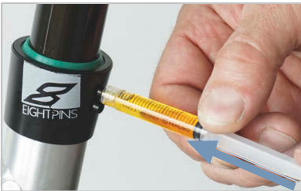
Figure 230: Lubricating the Eightpins seat post
