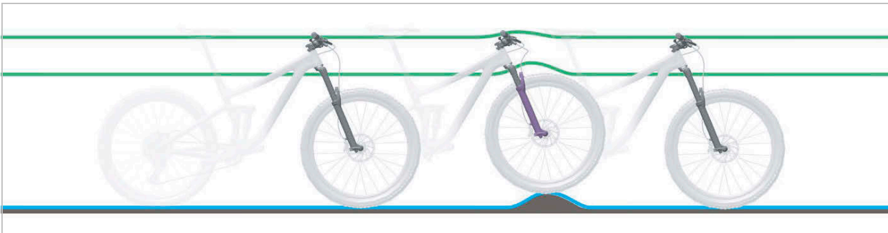
Figure 222: Compression damper set to hard and soft
