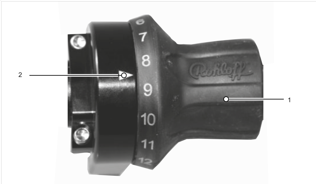
Figure 81: ROHLOFF gear shift
