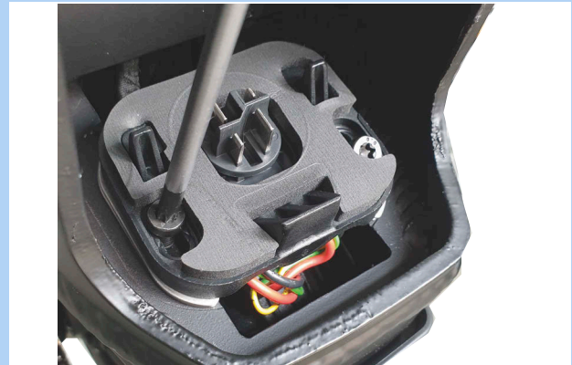
Figure 114: Undoing screws on battery mount
