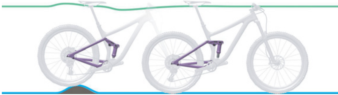
Figure 27: Optimum rear frame damper ride performance over bumps
