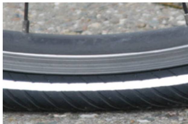
Figure 133: Much too little tyre pressure
