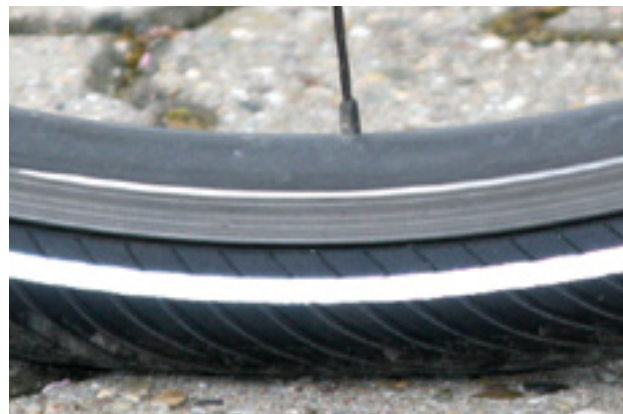
Figure 132: Correct tyre pressure. The tyre is barely deformed under the load of the body weight
