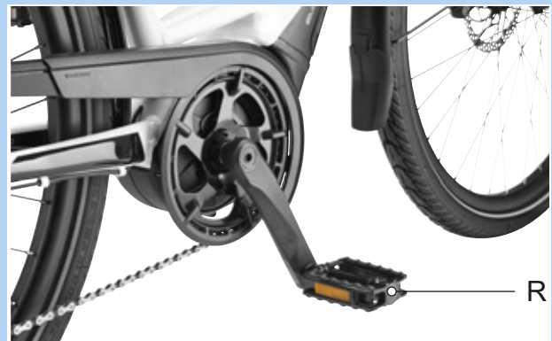
Figure 59: R-pedal in the right-hand crank arm
