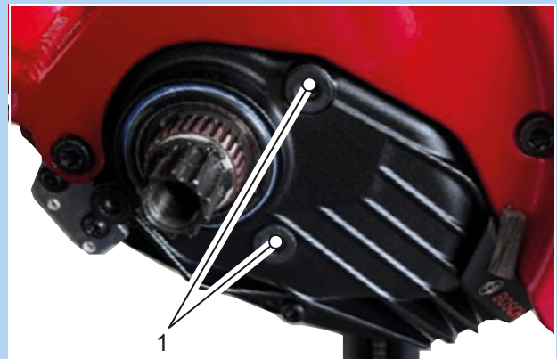
Figure 73: Position of attachment screws (1)
