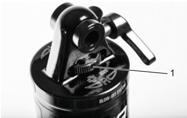
Figure 255: SR SUNTOUR rebound adjuster wheel (1) on the rear frame damper
