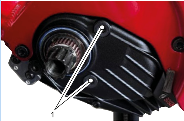
Figure 65: Position of attachment screws (1)
