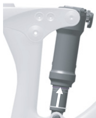
Figure 158: Moving the O-ring on the rear frame damper
