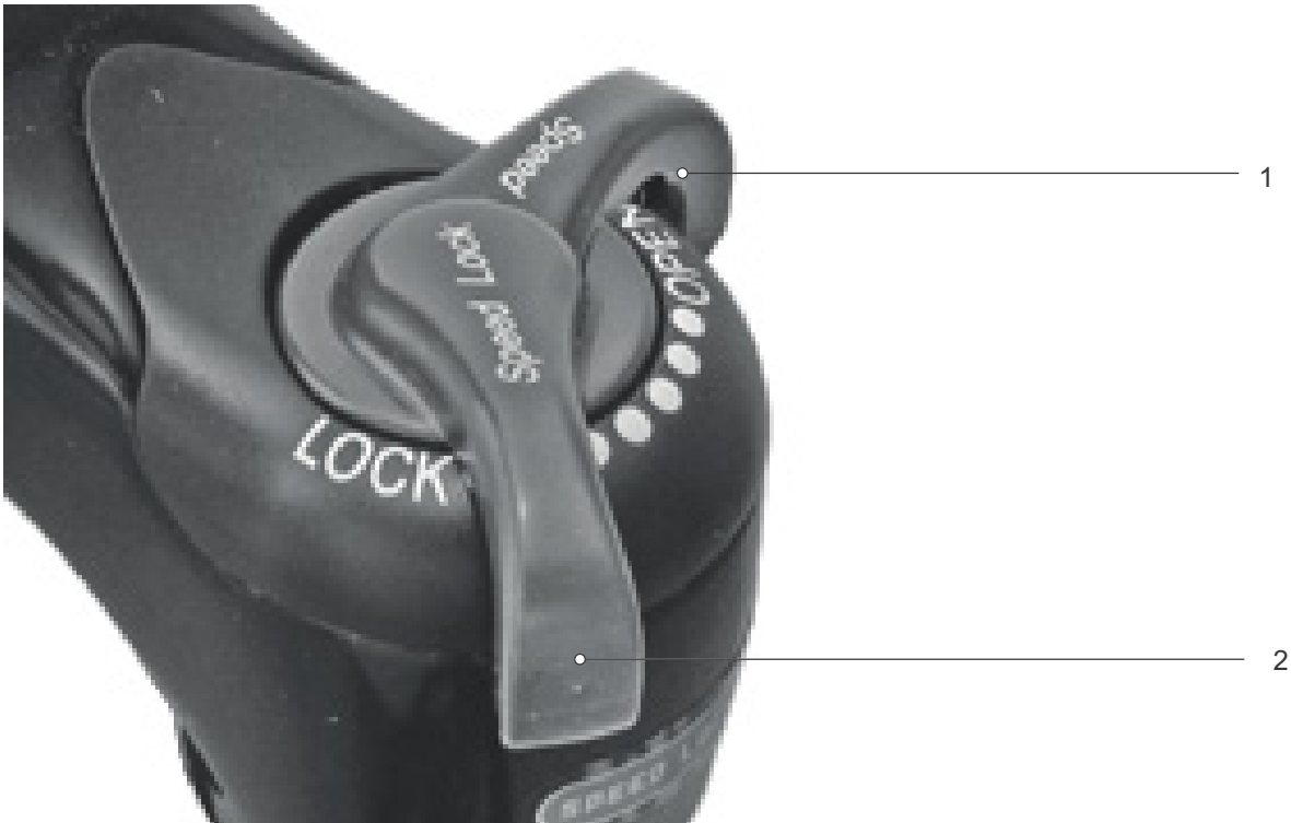
Figure 193: SR SUNTOUR compression adjuster in open (1) and closed (2) position
