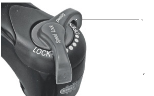
Figure 243: Changing compression adjuster to a harder setting
