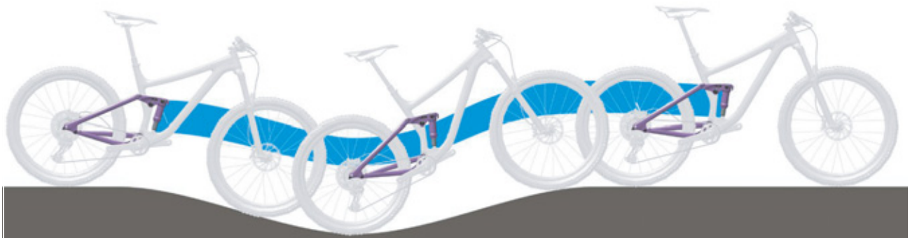
Figure 26: Optimum rear frame damper ride performance on hilly terrain
