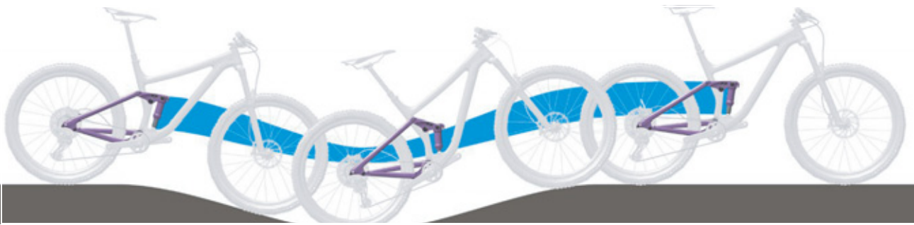
Figure 258: Excessively soft suspension in the rear frame damper on hilly terrain
