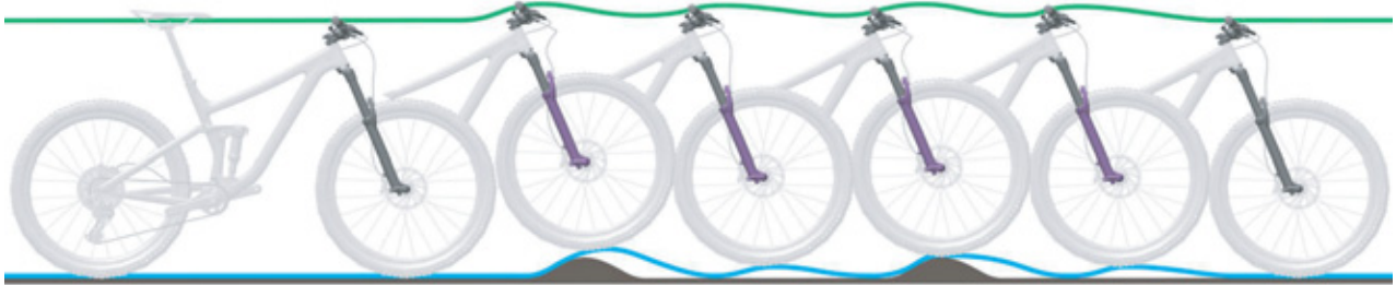
Figure 238: Suspension fork rebounding too quickly
