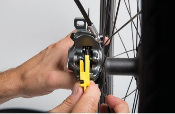
Figure 205: Checking the brake lining when fitted with the help of the transport safety wear gauge
