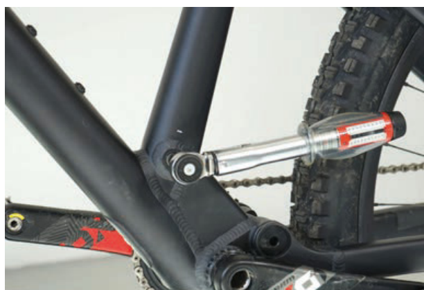
Figure 109: Tightening the seat post axle
