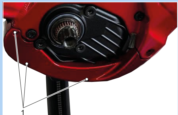
Figure 74: Attachment screws in lower motor cover (1)
