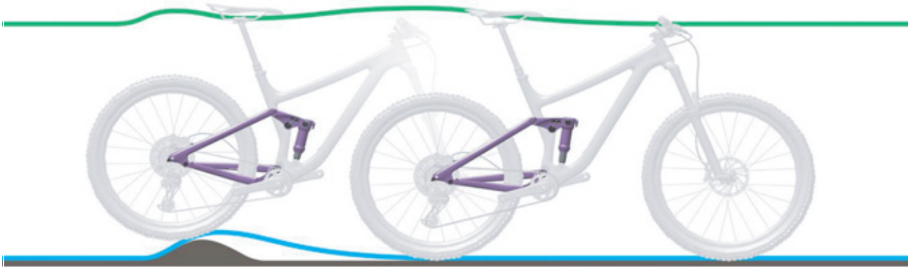
Figure 260: Excessively hard damping in the rear frame damper on bumps
