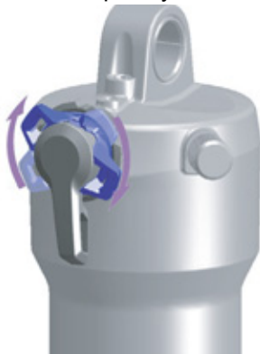
Figure 168: Changing compression adjuster to a harder setting
