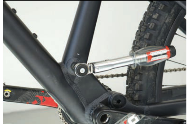
Figure 116: Tightening the seat post axle
