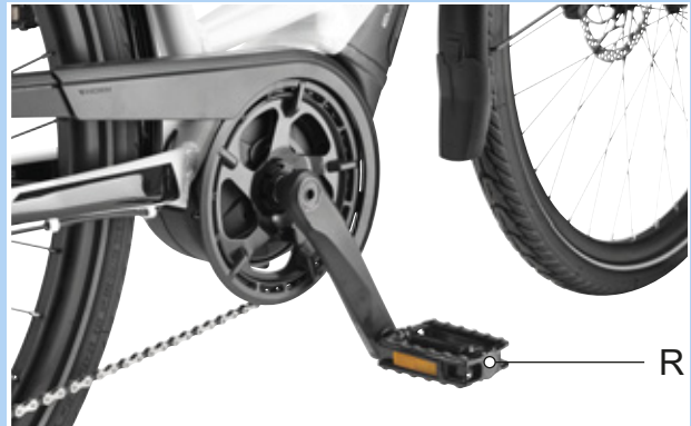
Figure 97: R-pedal in the right-hand crank arm
