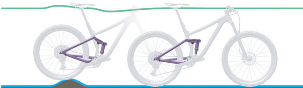
Figure 164: Optimum rear frame damper ride performance over bumps
