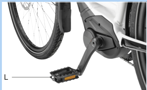
Figure 60: L-pedal in the left-hand crank arm
