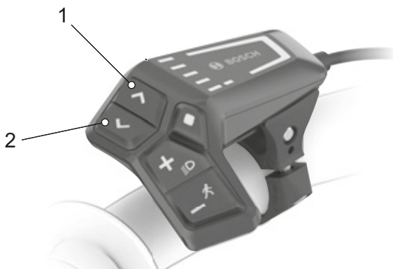
Figure 186: Position of increase brightness button (2) and decrease brightness button (1)
