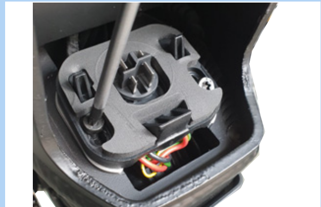
Figure 68: Undoing screws on battery mount
