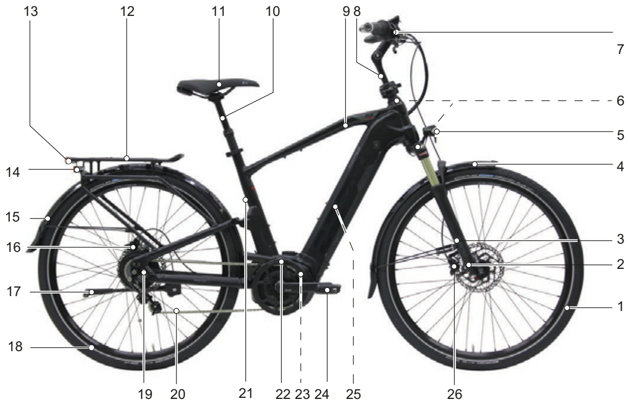
Figure 3: Pedelec viewed from right, Bull Cross Rider EVO 2 used as example
