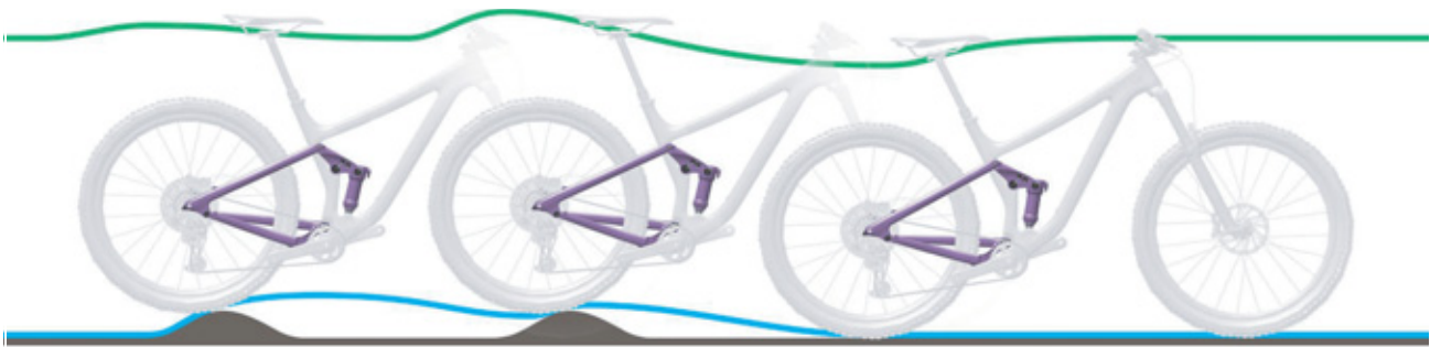
Figure 256: Rear frame damper rebounding too slowly
