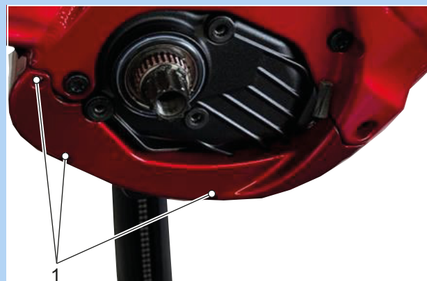
Figure 64: Attachment screws in lower motor cover (1)
