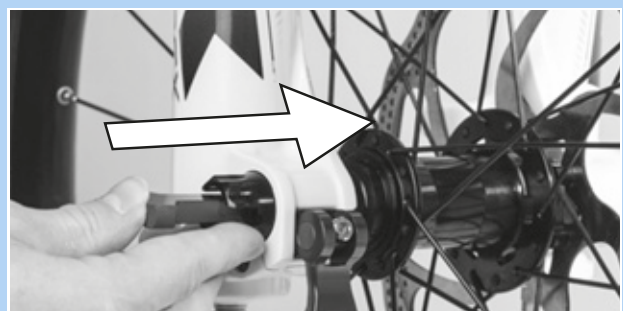
Figure 87: Pushing the red lever in the direction of the arrow
