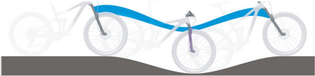
Figure 250: Excessively soft suspension in the suspension fork on hilly terrain
