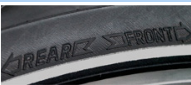
Figure 80: Rotation direction arrow on MTB tyres
