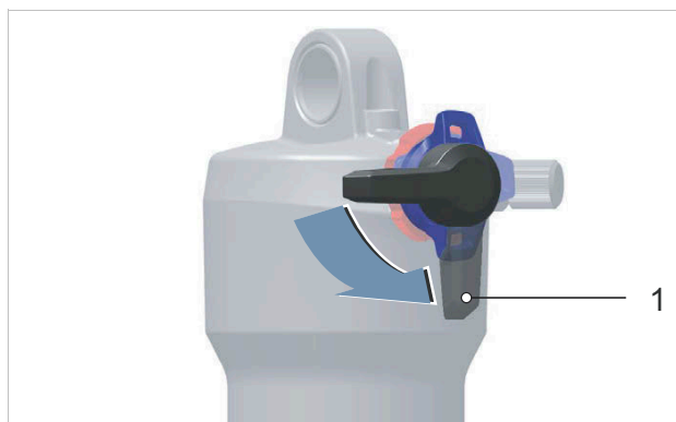
Figure 146: The compression adjuster's (black) open position (1)
