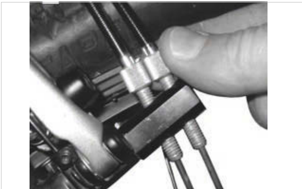
Figure 182: The tension adjuster on ROHLOFF hub versions with internal switch control is located on the tension counter support
