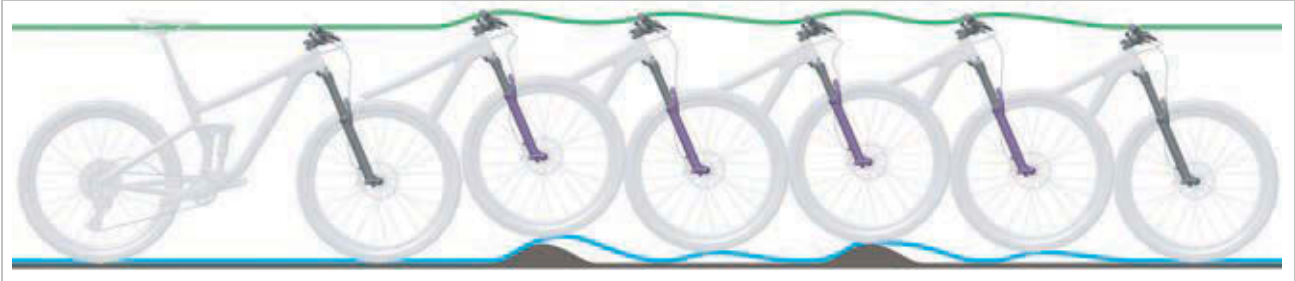
Figure 191: Suspension fork rebounding too quickly
