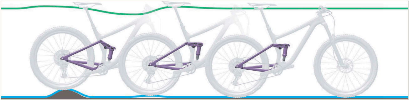
Figure 197: Rear frame damper rebounding too quickly
