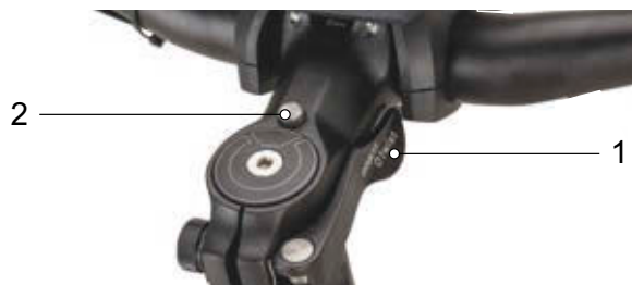
Figure 83: Stem, version II with clamping lever on the stem quick release (1) and unlocking knob (2)
