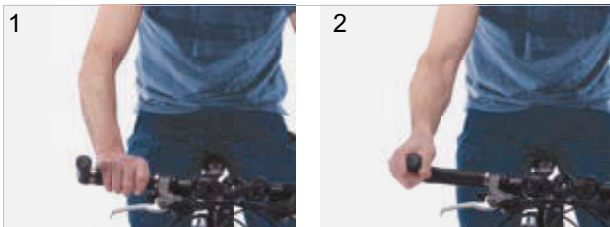
Figure 144: Grip positions on a bar end
