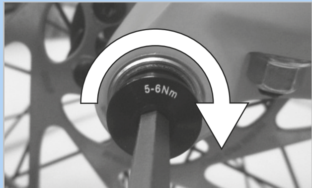
Figure 71: Tightening the securing screw
