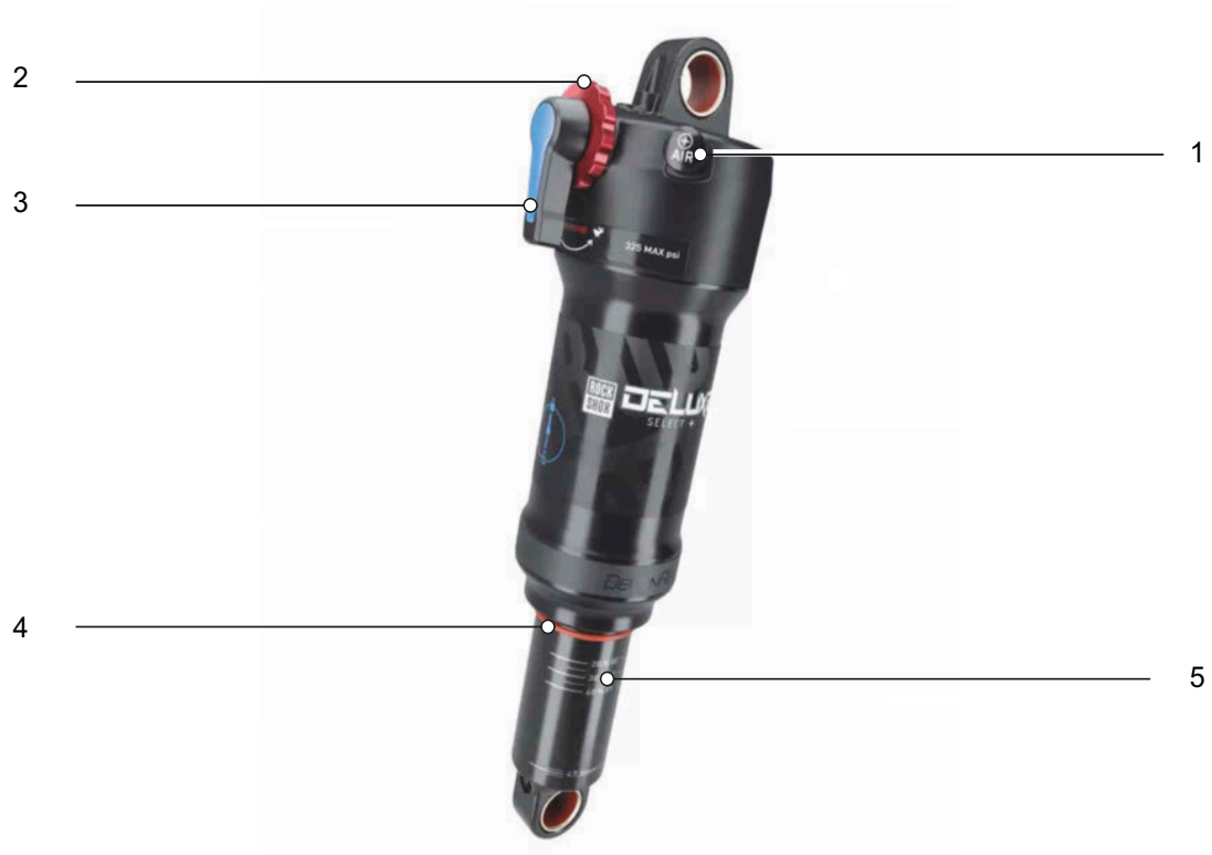
Figure 8: ROCKSHOX Deluxe Select rear frame damper structure design
