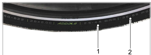
Figure 165: Tyre pressure specification in bar (1) and psi (2)
