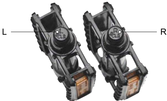
Figure 84: Example of markings on pedals
