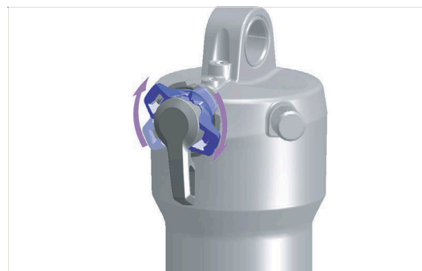
Figure 148: Adjust the compression adjuster so that it is harder
